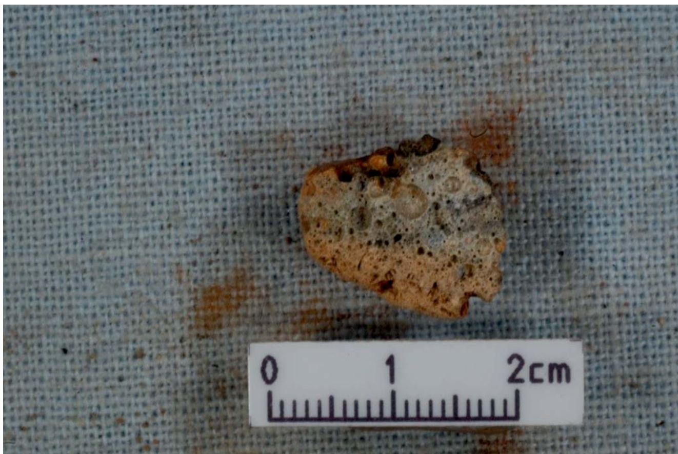
Plate 360. Fragment of part vitrified lightweight material interpreted here as heavily burnt daub (see Plate 358).
